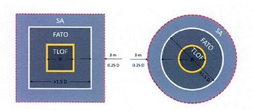
h) If a FATO is near a runway or taxiway and simultaneous operations are planned, the separation between the edges of the runway/taxiway and the FATO must meet the specified minimum distance:
